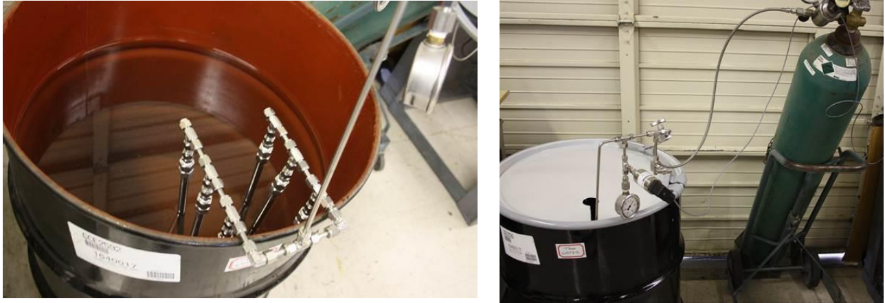
Figure 3: Picture of the setup used for the pneumatic proof test
