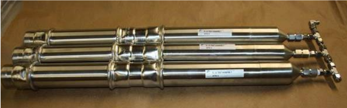
Figure 2: Picture of selected 2.0 in diameter specimens prior to the hydrostatic testing
