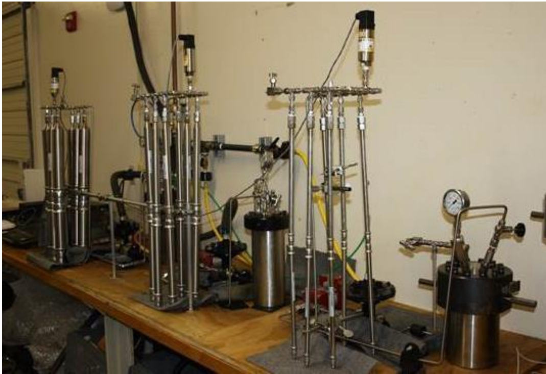
Figure 4: Picture of the setup used for the impulse test
