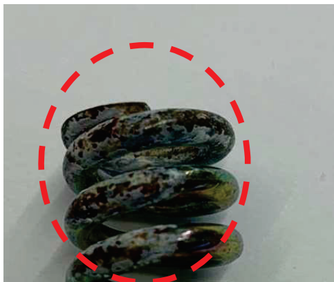
Competitor's PRV "Steel" Spring (corrosion shown)
